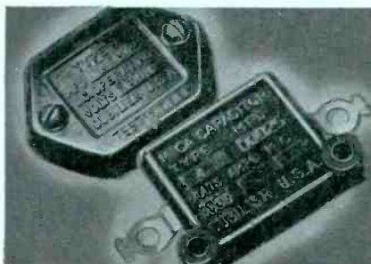
TYPES 9 AND 4 Mica Receiving-Transmitting Capacitors. Effectively used for R. F. bypass, high voltage D.C. blocking, low power tank capacitors, padders, coupling functions, audio and video purposes. Utilizing the exclusive C-D stack assembly process, these units are constructed of the finest India ruby mica and foil.
