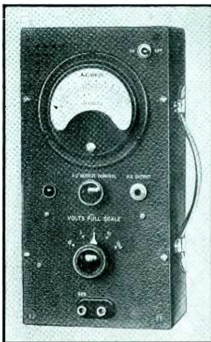
Fig. 1—Above. External view of the electronic voltmeter
