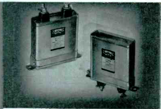
TYPE TJU Fireproof Dykanol Transmitting Capacitors. Dykanol (chlorinated diphenyl) impregnated and filled and hermetically sealed in sturdy steel containers. Supplied with adequate glazed porcelain or bakelite terminal (according to rating) insulators and universal mounting strap. Rigidly tested and conservatively rated.
